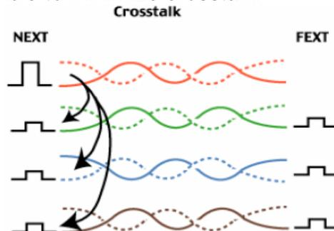
Cat 5e /6 testers measure crosstalk from one pair to all three other pairs for each pair and compare it to the 568 specs, giving a pass/fail result. Some also calculate "ACR" or attenuation/crosstalk ratio, as it is a measure of how big the crosstalk signal is to the
