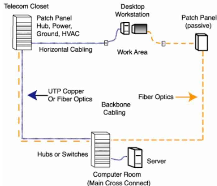
"568" calls for connecting the desktop (work area) to a telecom closet (the "horizontal" run) with up to 100 meters of cable (including no more than 10 m total of patchcords), which is usually Cat 3, Cat 5 or Cat5e UTP. The "Cat" or category designation refers to a performance grade, which we will explain later. Most copper installations today use Cat 5e or Cat 6 exclusively, as it isn't that much more expensive than Cat 3 and can support phones or any LAN on any outlet.
