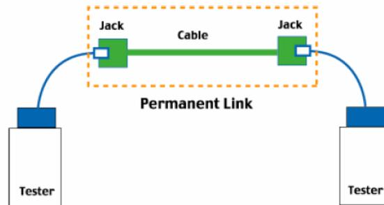
The tester's adapter interface cable may be the weakest link when testing. Conventional adapter cords may be the cause for many false failures in the field. Susceptible to the daily wear and tear associated with rough field conditions, they degrade with time and contribute to return loss.
