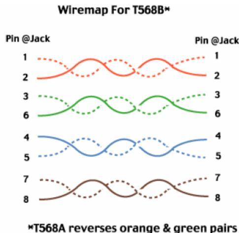
Most of the failures are simple enough to understand, like reversed wires in a pair, crossed pairs, opens or shorts. One possible failure, crossed pairs, is caused when both wires of a pair are crossed at one termination. The usual cause of a crossed pair is a 568A termination on one end and a 568B on the other.
