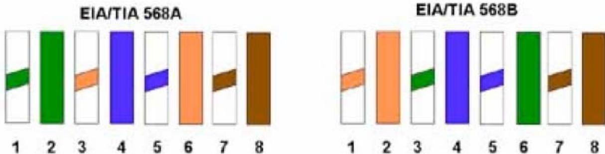
**Note:** Cat 3 jacks and all plugs are going to use these color codes shown above. However, Cat 5, 5e and 6 jacks have internal connections that continue the twists as close to the pins in the jacks as possible. Thus the pinout on the back of the jacks will not usually follow the standard color code layouts- see the pin sequence in the photo above and the twists in the internal connections of the jack here!
