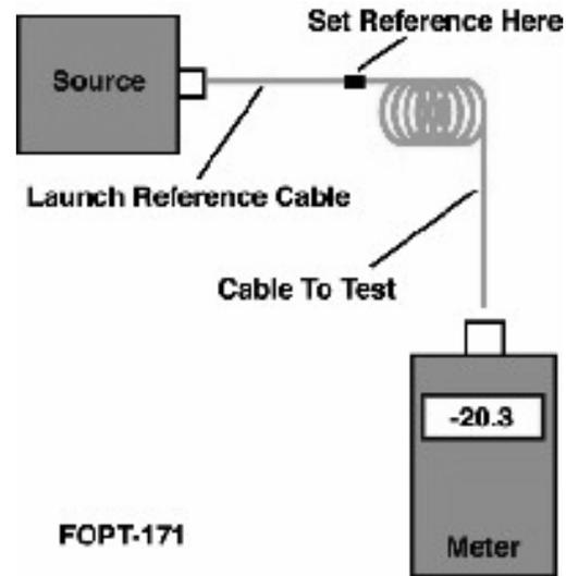
In a double-ended loss test, you attach the cable to test between two reference cables, one attached to the source and one to the meter. This way, you measure two connectors' losses, one on each end, plus the loss of all the cable or cables in between. This is the method specified in OFSTP-14, the test for loss in an installed cable plant.
