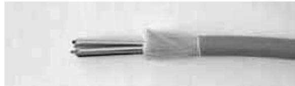
**Strength members:** Aramid fibers (Kevlar is the duPont trade name) used to pull the cable. The term is also used for the fiberglass rod in some cables used to stiffen it to prevent kinking.
