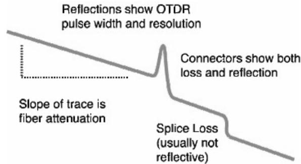
OTDRs can also detect problems in the cable caused during installation. If a fiber is broken, it will show up as the end of the fiber much shorter than the cable or a high loss splice at the wrong place. If excessive stress is placed on the cable due to kinking or too tight a bend radius, it will look like a splice at the wrong location.
