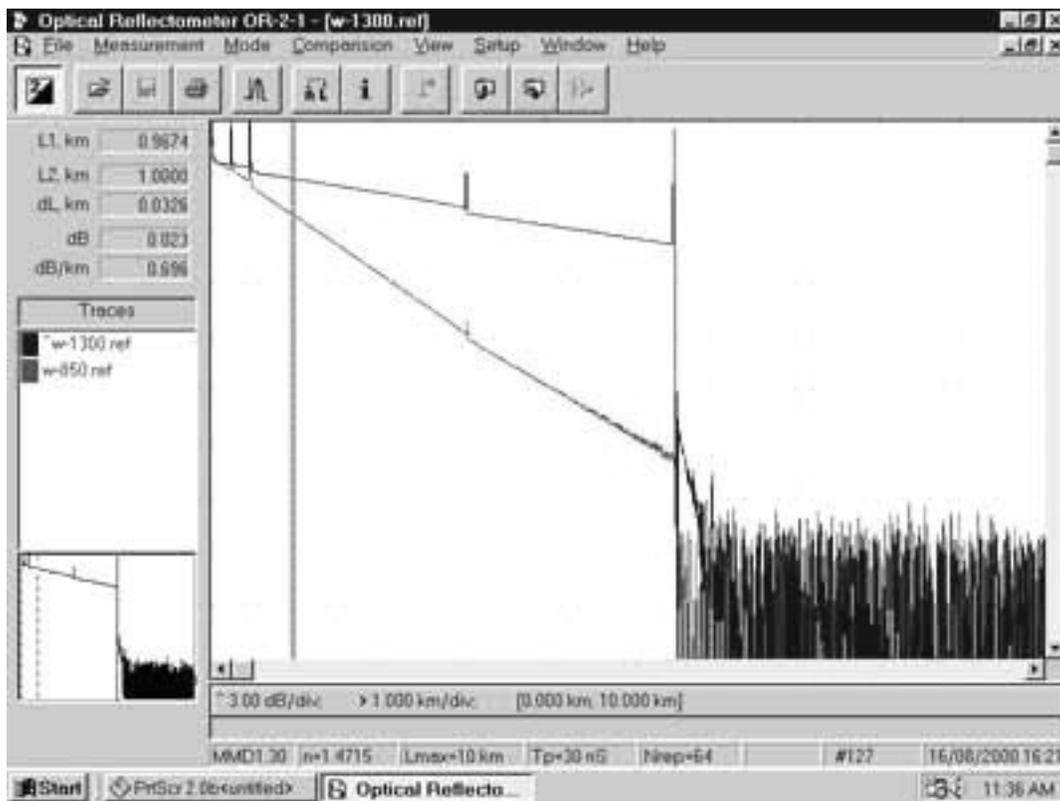
There is a lot of information in an OTDR display. The slope of the fiber trace shows the attenuation coefficient of the fiber and is calibrated in dB/km by the OTDR. In order to measure fiber attenuation, you need a fairly long length of fiber with no distortions on either end from the OTDR resolution or overloading due to large reflections. If the fiber looks nonlinear at either end, especially near a reflective event like a connector, avoid that section when measuring loss.
