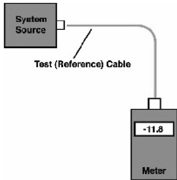
To measure power, attach the meter to the cable that has the output you want to measure. That can be at the receiver to measure receiver power, or to a reference test cable (tested and known to be good) that is attached to the transmitter, acting as the "source", to measure transmitter power. Turn on the transmitter/source and note the power the meter measures. Compare it to the specified power for the system and make sure it's enough power but not too much.
