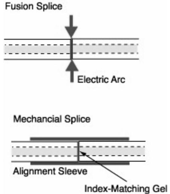
Fusion Splices are made by "welding" the two fibers together usually by an electric arc. Obviously, you don't do that in an explosive atmosphere (at least not more than once!), so fusion splicing is usually done above ground in a truck or trailer set up for the purpose. Good fusion splicers cost \$15,000 to \$40,000, but the splices only cost a few dollars each. Today's
