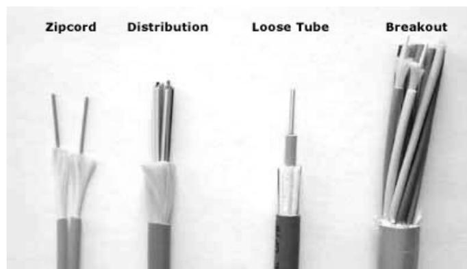
**Simplex and zip cord:** Simplex cables are one fiber, tight-buffered (coated with a 900 micron buffer over the primary buffer coating) with Kevlar (aramid fiber) strength members and jacketed for indoor use. The jacket is usually 3mm (1/8 in.) diameter. Zipcord is simply two of these joined with a thin web. It's used mostly for patch cord and backplane applications, but zipcord can also be used for desktop connections.
