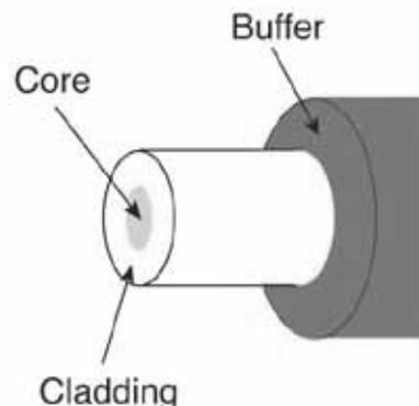
**Multimode fiber:** has a bigger core (almost always 62.5 microns - a micron is one one millionth of a meter - but sometimes 50 microns) and is used with LED sources at wavelengths of 850 and 1300 nm for short distance, lower speed networks like LANs.
